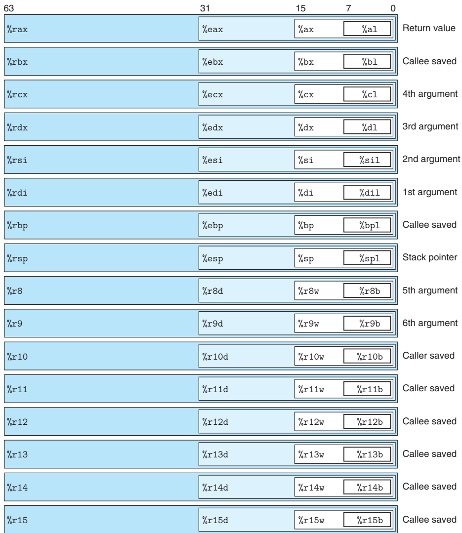
Figure 3.2 Integer registers. The low-order portions of all 16 registers can be accessed as byte, word (16-bit), double word (32-bit), and quad word (64-bit) quantities.
