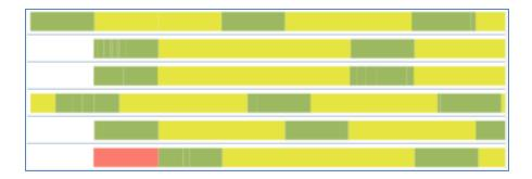
In this screenshot, each horizontal band represents a thread, with time on the x-axis. Green is execution time, red is time spent blocked, and yellow is time where the thread could have run but was preempted by another thread. The more yellow there is, the more oversubscription there is hurting performance.
