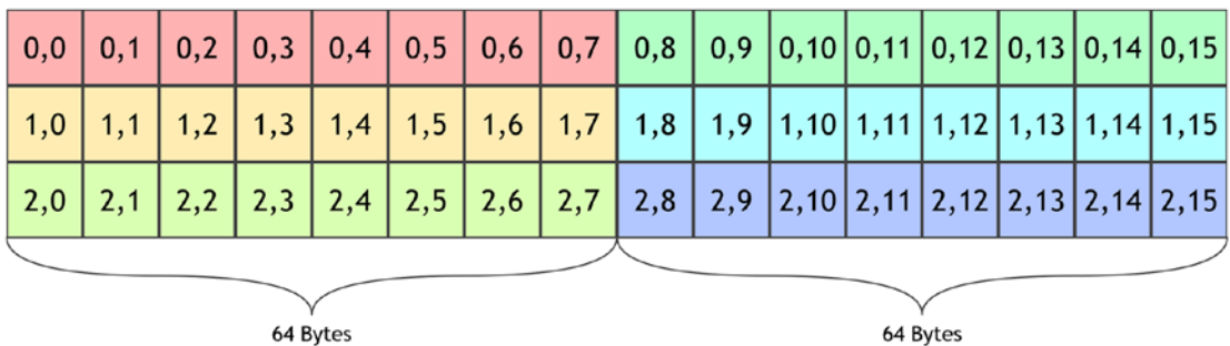
Figure 8-1. Square array and CPU cache lines
